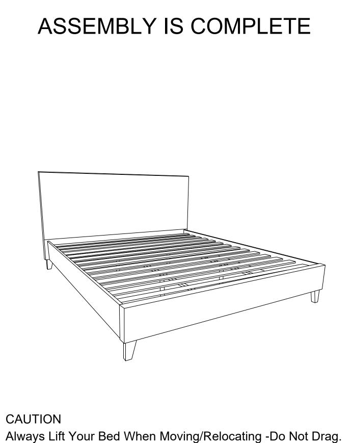
Dragging Can Cause The Centre Support Legs To Bend/Break
